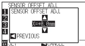
11 Press the POSITION (▲▼) key and increase or decrease the setting value. Set the X value measured in step 9.
