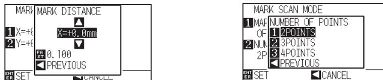
Increase or decrease the setting value using POSITION (▲▼) key. Select the change unit by [FAST] key.
