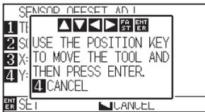
7 Press the POSITION (▲▼◀▶) key and move the tool carriage to the area to start scanning of the registration mark.
