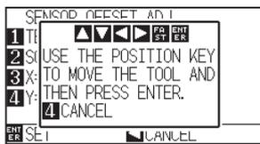
8 Press the POSITION (▲▼◀▶) key and move the tool carriage to the position to plot the registration mark (position nothing is printed).
