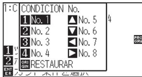
2 Presione la tecla [1] (No.1), la tecla [2] (No.2), la tecla [3] (No.3), la tecla [4] (No.4), la tecla [▲] (No.5), la tecla [▼] (No.6), la tecla [◀] (No.7) o la tecla [▶] (No.8), presionando simultáneamente la tecla [ENTER].
