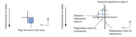
Using the registration mark plotted in step 9, measure the distance of how much the adjustment registration mark needs to be moved so both will overlap, and record the value. As an example, in the figure above, it needs to move in negative directions for both X and Y directions, so both of the adjustment values will be negative values.
