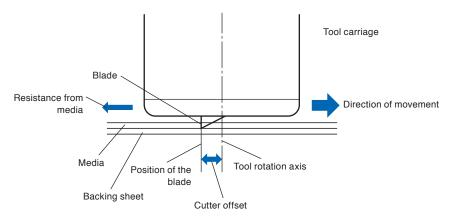
The blade tip gets sunk into the media with 0.3 mm or thicker, making the blade hard to rotate. Especially for the corners where two straight lines meet, cutting becomes very hard because it cannot rotate smoothly.
