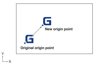
Press the POSITION (▲▼◀▶) keys to move the tool to the new origin point.
