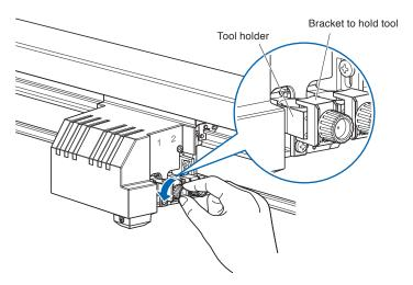
2 While pushing up the tool holder, push the tool into the holder until its flange completely touches the upper part of the holder.
