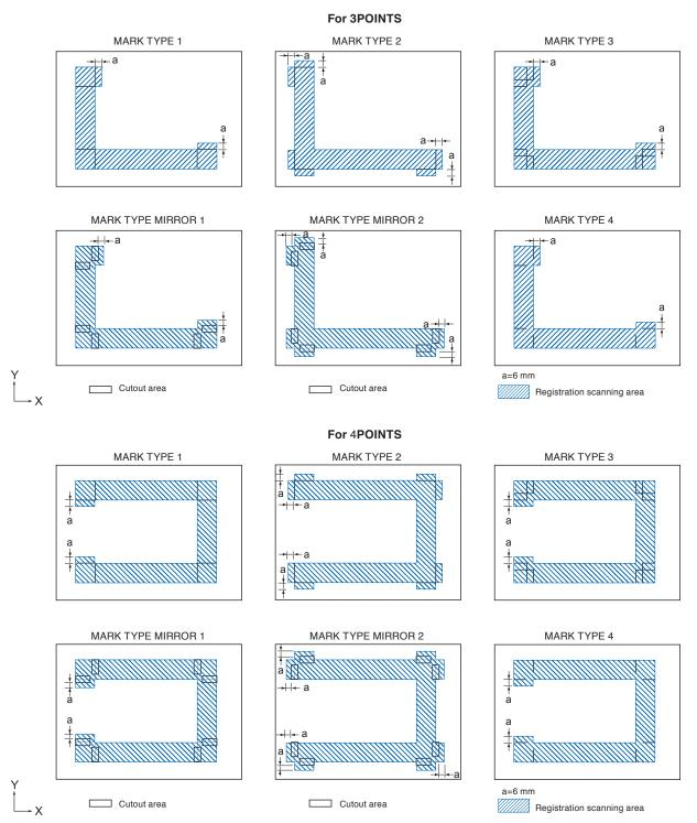
The area necessary to scan the registration mark when the Mark Distance is set is as following: Do not print in the shaded area shown in the Figure below.
