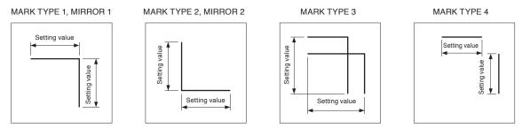
When the registration marks are sensed, it will start from the lower left registration mark on the document, and sense the next registration mark in the horizontal and vertical direction.
