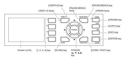
This section explains the function of lamps and keys on the control panel.
