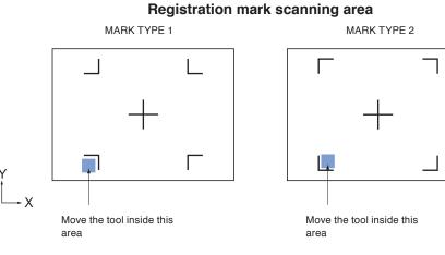
9 Confirm the position of the tool and press the [ENTER] key.
