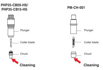
2 Attach the plunger cap after the cleaning is finished.
