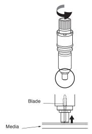
2 Extend the blade little by little to the thickness of the media. Optimal blade length is less than the thickness of film and backing sheet combined, but more than the thickness of the film.
