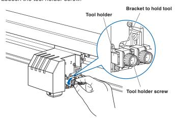
2 While pushing up the tool holder, push until the flange of tool completely touches the upper part of the holder.
