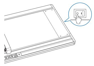
2 Connect one end of the provided power cord to the FCX4000 AC line inlet and the other end to an electrical socket of the rated supply voltage.
