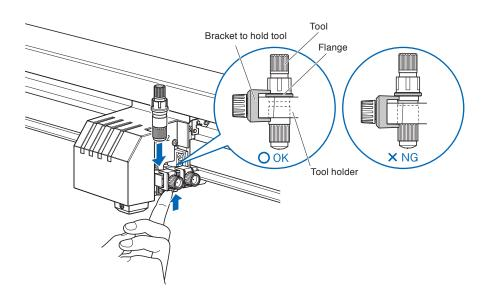
*3* Make sure that the tool bracket is engaged on the tool's flange, and then tighten the screw.
