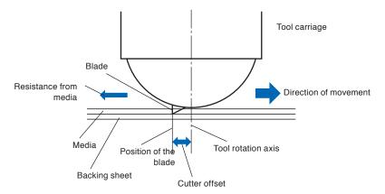
The blade tip gets sunk into the media with 0.3 mm or thicker, making the blade hard to rotate. Especially for the corners where two straight lines meet, cutting becomes very hard because it cannot rotate smoothly.
