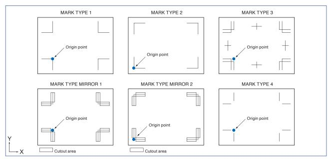
The origin point after scanning the registration mark will be as shown below.
