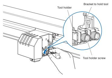
2 While pushing up the tool holder, push the tool into the holder until the flange of tool completely touches the upper part of the holder.
