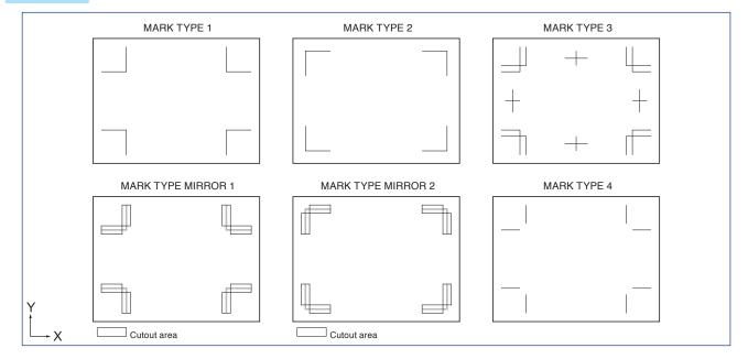
With more registration marks, precision of matching the printed image and the cutting will increase. But if there are many registration marks, it will take longer to sense, and the area that can be cut becomes smaller.
