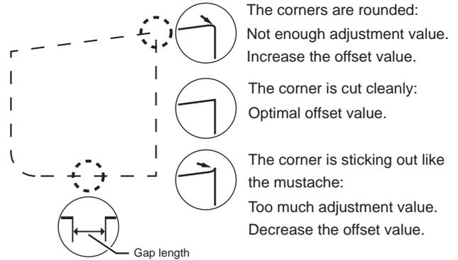
When the gap length is not enough, those the gap area is torn and may come off during cutting.
