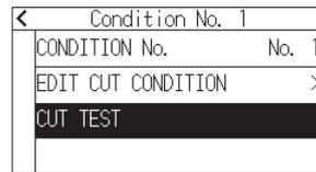
Check the result of the test cut and adjust the SPEED, FORCE, ACCELERATION and GAP LENGTH to the optimum value. The optimal length is slightly greater than the thickness of the media. Adjust the offset value and gap length if the corner is not cut or if it is cut too much.
