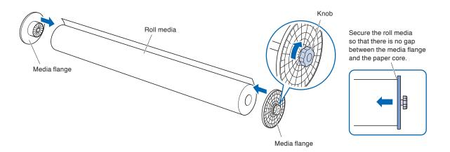
3 Load the roll media on the stock shaft so that the tip of roll media is facing upward.
