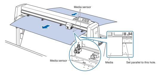
3 Position the media and the push rollers to correspond with the width of the media.
