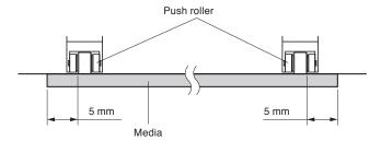
6 Pull the media taut to make sure that there is no slack in the conveyance path, and then raise the media set lever to lower the push rollers.
