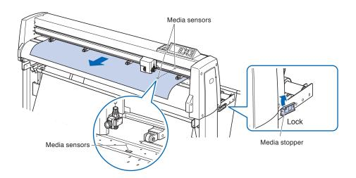
Position the media and the push rollers to correspond with the width of the media.
