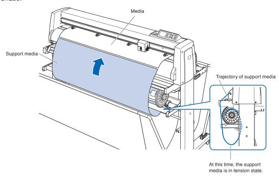
Stick and secure the loaded roll media and the support media using tape.
