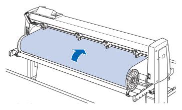
5 Lock the media stopper (Raise while pulling forward) and pull it out evenly so that the roll media is straight. Please load so that the roll media always rests on the media sensor.
