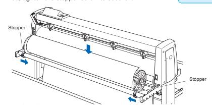
4 Push the tip of the roll media forward from the back of the FC9000. Make sure to pull it so that there is no slackening across the roll media's route.
