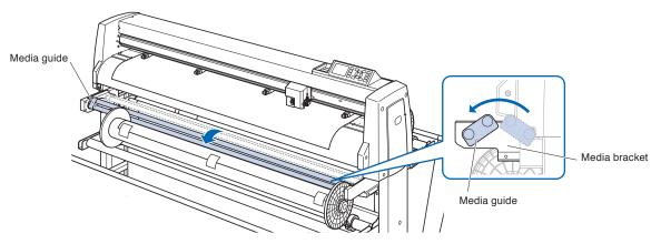
Pull up the support media to the machine's cutting mat surface.
