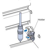
Once the pen is attached, releasing the holder fixes the pen in place.
