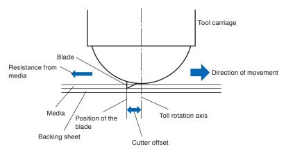
The blade tip gets sunk into the media with 0.3 mm or thicker, making the blade hard to rotate. Especially for the corners where two straight lines meet, cutting becomes very hard because it cannot rotate smoothly.
