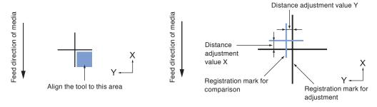
Using the registration mark plotted in step 9, measure the distance of how much the adjustment registration mark needs to be moved so both will overlap, and record the value. As an example, in the figure above, it needs to move in negative directions for both X and Y directions, so both of the adjustment values will be negative values.
