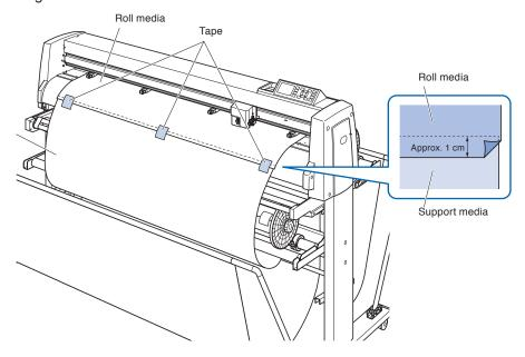
**9** After securing with tape, feed the roll media to a position where the overlapping portion between the roll media and support media does not overlap the media guide, and set that position as the origin.
