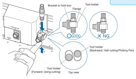
3 Make sure that the tool bracket is engaged on the tool's flange, and then tighten the screw.
