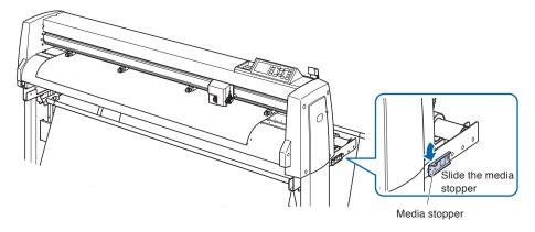
When the set lever is up (and the media is held down by the push rollers) and the media stopper is unlocked, pull out the roll media and give it slack.
