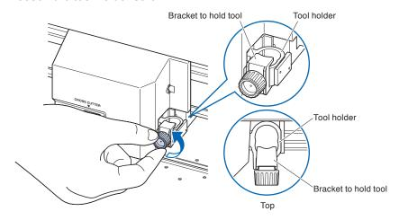
While pushing the tool holder in the upward direction, push the Pouncing tool all the way into the holder until its flange contacts the upper part of the holder. The flat edge must be parallel to the tool holder.
