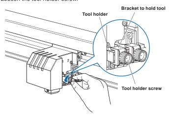
While pushing up the tool holder, push until the flange of tool completely touches the upper part of the holder.
