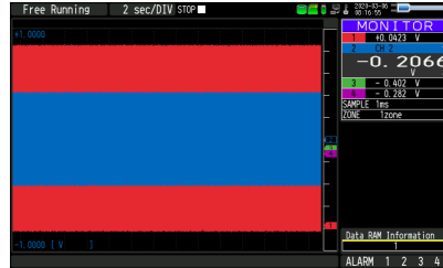
CH2 is active CH. The waveform of CH2 is displayed on the top, so you can visually recognize it.
